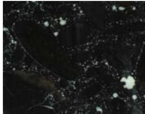
*Concrete specimen prepared for void analysis. The voids have been filled with oxide (white) and the matrix has been inked (black).*
